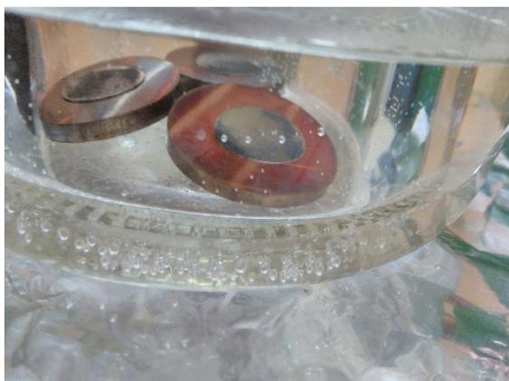
**Figure 4.**  $\text{Li}_3\text{N}$  coated Li chips.
