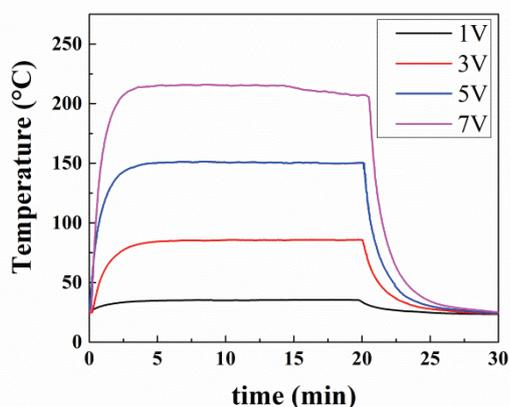
**Figure 3.** Time dependent heating behavior of 15 nm Al<sub>2</sub>O<sub>3</sub> deposited copper nanowire thin film under different applied voltages.
