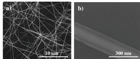
**Figure 1.** SEM images of (a) bare copper nanowire network and (b)  $\text{Al}_2\text{O}_3$  deposited copper nanowire.
