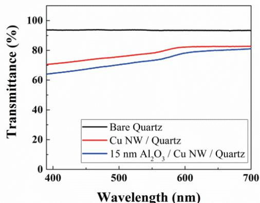
**Figure 2.** Transmittance of bare and Al<sub>2</sub>O<sub>3</sub> deposited copper nanowire thin films. Transmittance of bare quartz is also provided for comparison.
