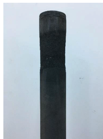
Figure 2. The graphite anode without alumina cover used in the early experiments
