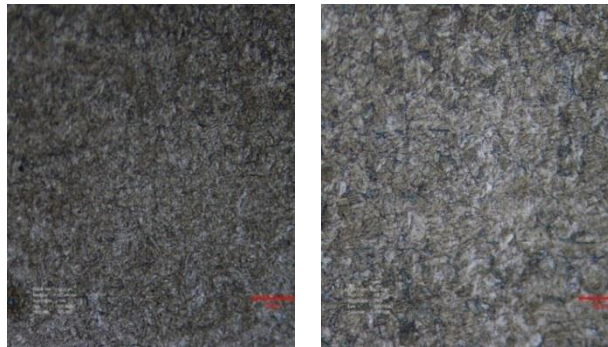
a) Carburized sample (Case) b) Carburized sample (Core)
