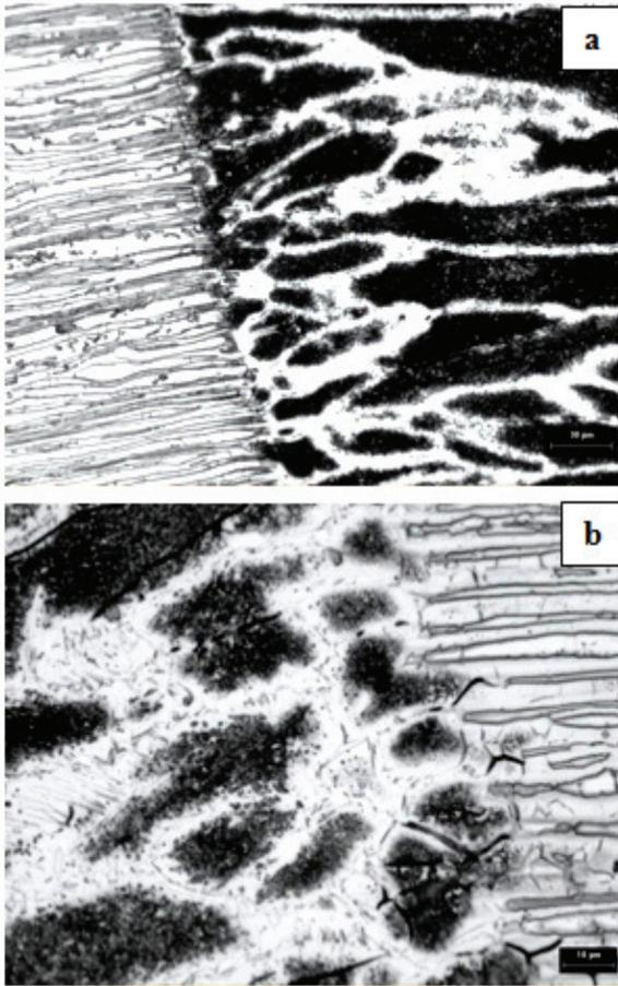
**Figure.1.** Microstructure of laser welded joint, a) HAZ (200X), b) HAZ (500X)
